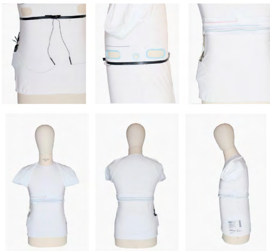
Fig.7 Smart&Safe Smart T-shirt, details. Focus on wearable add-on Smart T-Shirt. Focus on arrangement of conductive yarns by color and type of sensor connection; study of electronics components to operation and monitoring of vital parameters. Source: Smart&Safe Project, 2020
