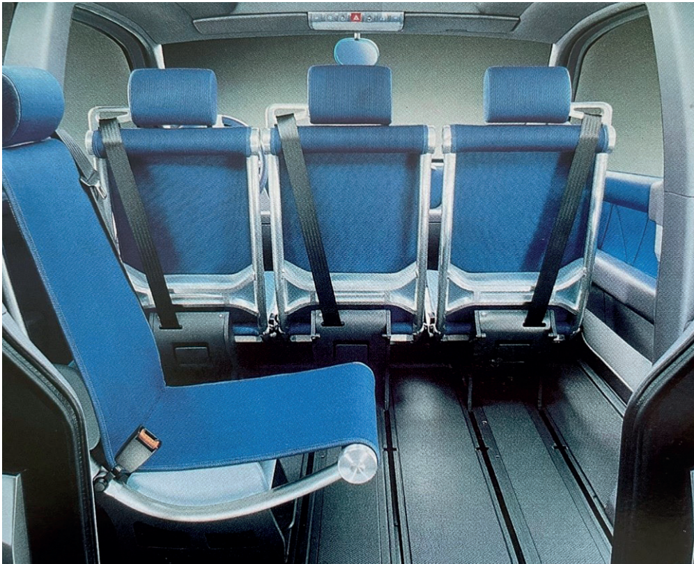
Fig. 5 - P3: Modular Seat Concept and Sliding Seats Note. Source: Adapted from (Barufaldi, 1999, p. 23)
